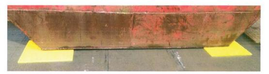
The mats are lightweight and can be easily manoeuvred. Salt water, water, oil, kerosene, drilling fluid and oil based mud tests have been carried out on the product with it showing no wear or absorption of the chemicals.
